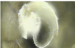
FAILED CIPP LINER
