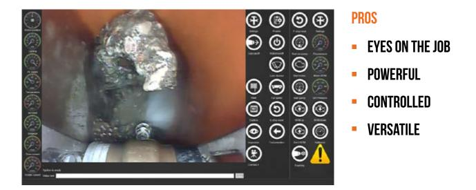
Eyes on the job and continuous adjustment of water pressure, angle with the pipe and distance to the material enable the operator to achieve the breakdown and elimination of various obstructions without adding damage to the pipe structure.
