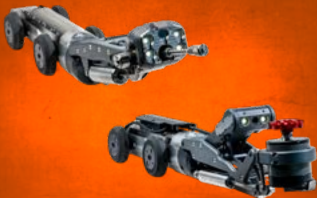
UPGRADED TO UHP WATER JET AND CUTTER
